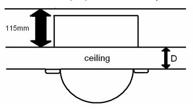
2. Take away the 3pcs leaf springs inside the accessory box. Attach the springs onto the outer cover. According to thickness of ceiling to adjust the location of springs. Find springs directions as following photo:
